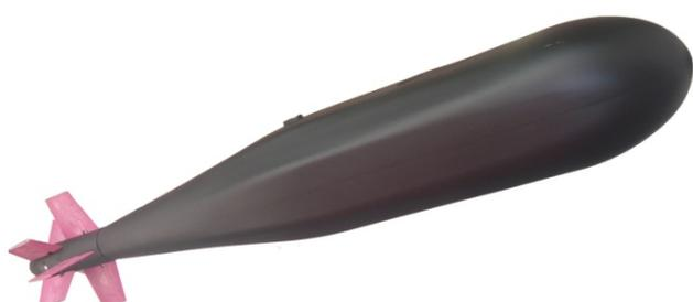
Flamingo (Forest Flames Intelligent Outputter) is an intelligent civil bomb. It is launched in groups from any cargo aircraft at a safe altitude; they individually glide and seek their targets along the fire front with the aid of GPS and other sensors contained in a recyclable control unit. Each Flamingo also has a single-use deposit with 200 liters of optimized retardant to extinguish the fire.
